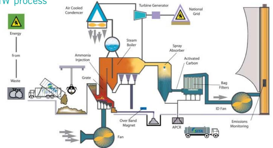
The plant and the entire treatment process are designed for maximum efficiency and safety.
