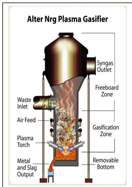
One diagram, entitled the Alter Nrg Plasma Gasifier, shows a “Syngas Outlet” but it is not attached to anything. In actual operation, this would be attached to piping that takes the syngas to the combustion/incineration device (an industrial boiler or internal combustion engine) and then to a stack that would emit dioxin and other pollutants into the air.
