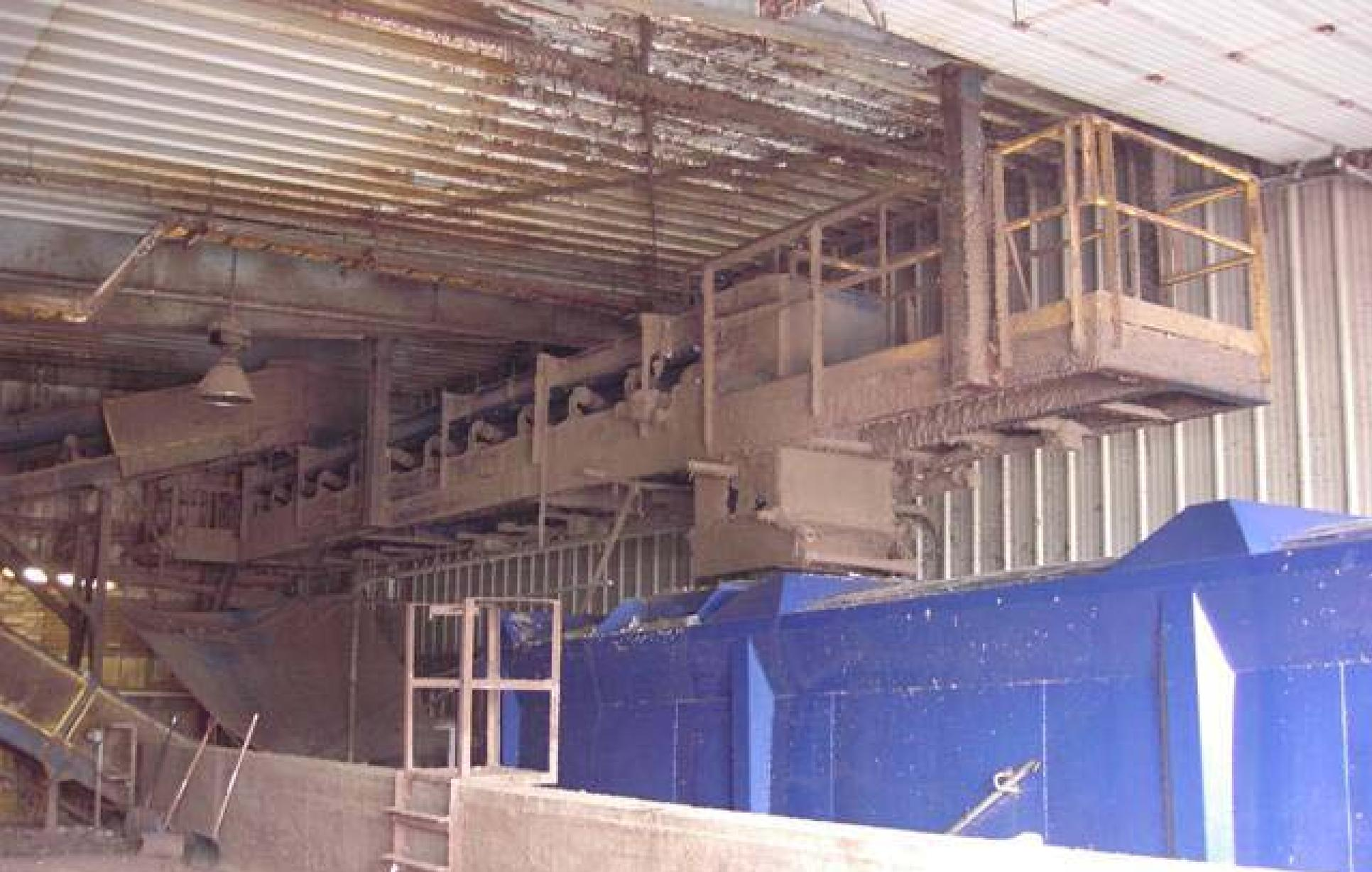
**Stabilized waste loaded by conveyor into transfer trailer**
