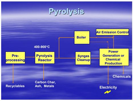
The solid byproducts from pyrolysis are mainly carbon char and non-thermally degradable materials such as silica (sand), metals, and glass. In the case of low temperature pyrolysis, a liquid fuel (tars and oils) may be produced. The metals can be separated from the char for recycling. The ash is usually disposed of in a non-hazardous landfill.
